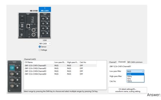
unfortunately, there isn't any alternative method to filter at 200Hz since the filter is on the hardware side of thing.
